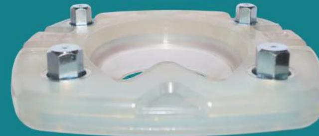
When screwed into a Duplo model with ring-shaped metal inlay, the stud sinks into the thread insert for about 3mm. That way, the first pitch of the screw thread won't be damaged even during abrasion and the thread will be easier to clean.
