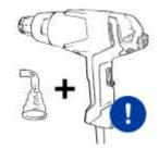
**CAUTION** Ensure that your hot air tool is switched off and, ideally, unplugged while attaching the reduction nozzle.
