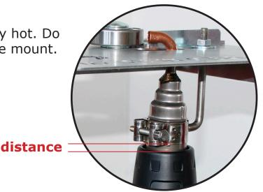
You can also vary the position of the hot-air gun on the upper side of the welding board. Use the combination spanner wrench 13mm (no. **2**) to unfasten the nut. Reposition the hot-air gun along the hole and re-tighten the nut hand-tight.
